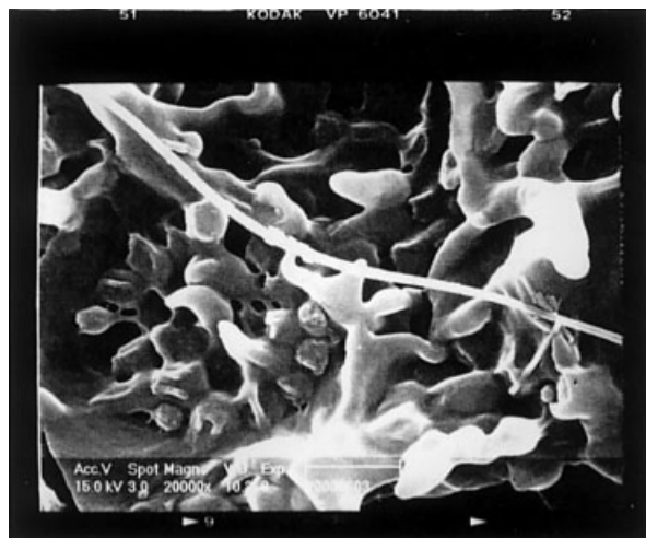
Figure 7 SEM photograph of EVA deformation.
